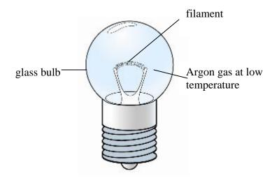
Oxygen in the glass bulb is vacuumed out and an inert gas such as argon is put in to prevent the tungsten filament from burning out.
