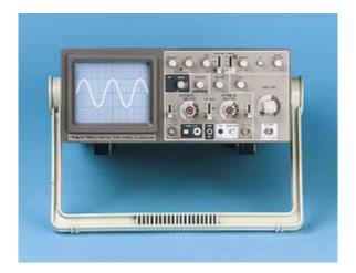
A cathode-ray oscilloscope, abbreviated CRO, or just called a scope, is a modern electronic test equipment that allows signal voltages to be displayed on a screen. The screen actually displays a graph of potential difference on the vertical axis against time on the horizontal axis.
