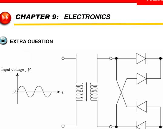
With four diodes arranged in a rectification circuit as shown, can you draw the output voltage,  $V_{\rm R}$ , on the graph given?
